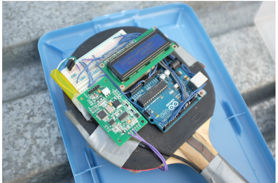
TOOLS OF THE TRADE | A homemade RFID scanner (invented by Quentin Caudron and Romain Garnier) used by Graham's group to identify tagged mice on the farm.
