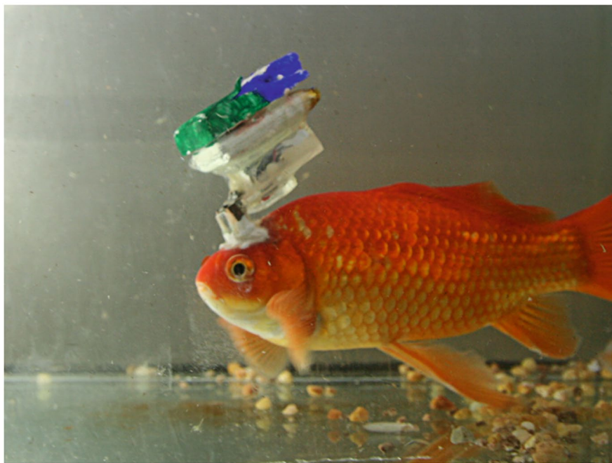
To better understand 3D navigation under water, it’s possible to capture electrophysiology data from swimming fish. The colored Styrofoam block adds buoyancy. Credit: Segev lab, Ben-Gurion Univ. of the Negev
