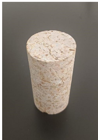
Figure 3. Sample of mildly weathered granite.
