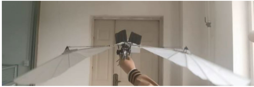
Figure 18. Passive deformation of wings flapping with sinusoidal speed regulation in downswing stage of the ornithopter.
