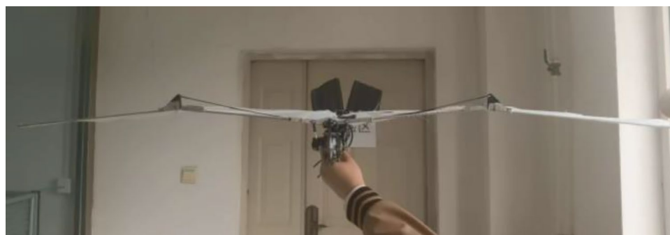
Figure 17. Passive deformation of wings flapping with sinusoidal speed regulation in baseline scenarios of the ornithopter.
