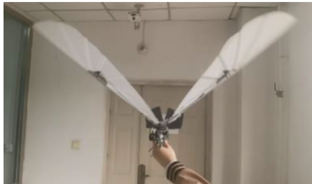
Figure 19. Passive deformation of wings flapping with sinusoidal speed regulation in upswing stage of the ornithopter.
