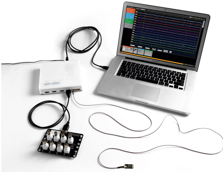
A simple set up: The Open Ephys acquisition board, shown with Intan headstage and laptop. Credit: J. Henkel. Reprinted with permission from Siegle et al. J Neural Eng 14 , 045003 (2017)
