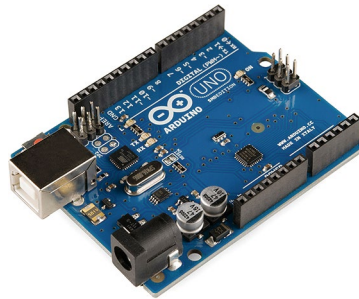
Staples gone micro: Arduino microprocessors (pictured) and Raspberry PI microcomputers are inexpensive hardware options. Credit: SparkFun Electronics
