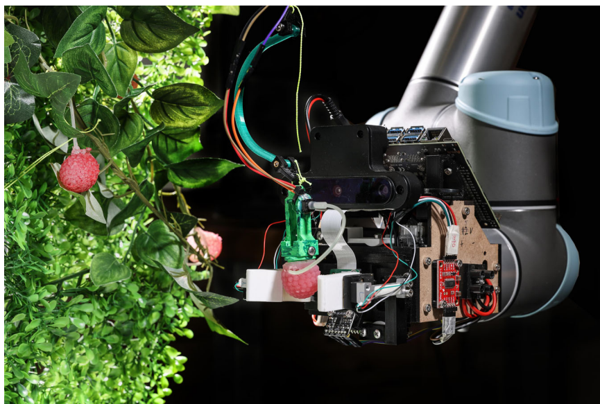
Fig. 2 Photograph of the physical twin of Raspberry and robot in training (credit: Kai Junge, Alain Herzog).
